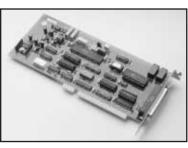
The ADC-16's high-precision current source has a compliance of –10V to +4V. This source can be used to directly excite resistance-based transducers such as RTDs.
